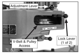
**Figure 29.** Model G0747 V-belt and pulleys exposed.
